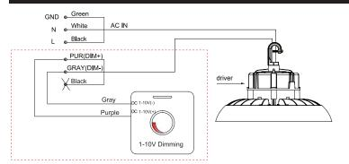
Turn off the power, connect AC wire. black wire to L, white wire to N, and green wire to E.
