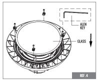
Put the glass cover back on the fixture using alen key and the clips and screws, tighten it.
