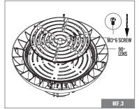
Fix the 60 or 90 degree lens to the board using the 3 pieces M3\*6 screws.
