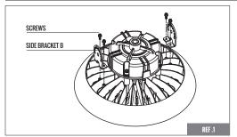
Fix the 2 side brackets B on each side using provided screws.
