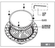
Place the fixture upside down, use an alen key to loosen the screws and clips that holds the glass cover. Remove the glass cover and the aluminum reflector.
