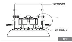
Assemble the yoke bracket A with the side bracket B as show in the figure.
